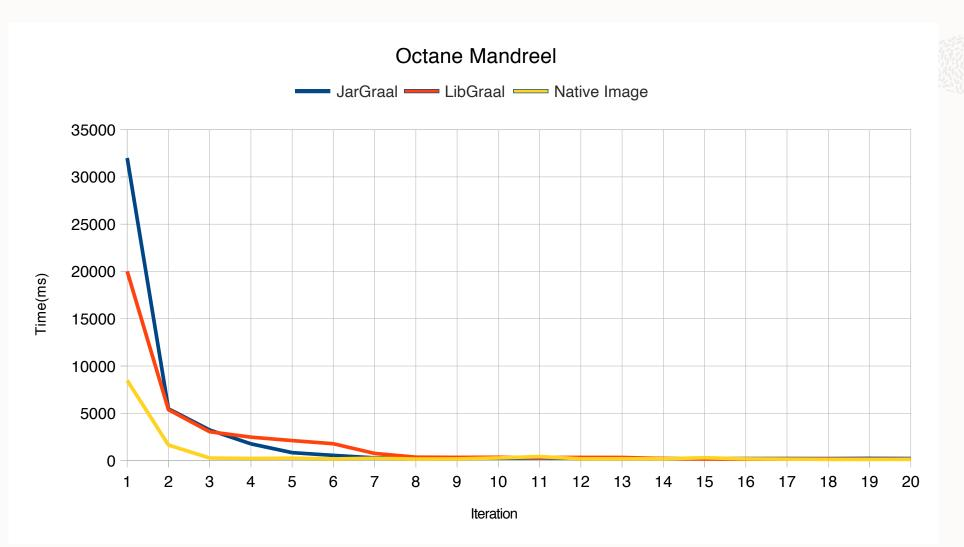
Time of each iteration running Octane Mandreel Times are average values of 10 executions 100 iterations time reduced from 47,60s to 41.6s
