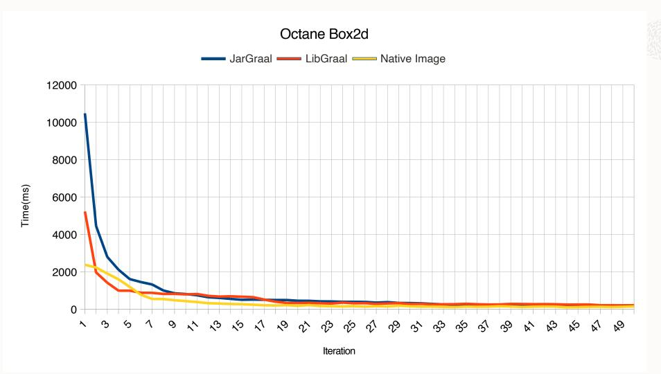
Time of each iteration running Octane Box2d Times are average values of 10 executions 100 iterations time reduced from 58,58s to 35,83s
